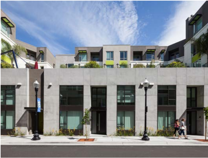
Example: Increased ground-floor to finished ceiling height in non-residential use areas increases the flexibility of these spaces.
